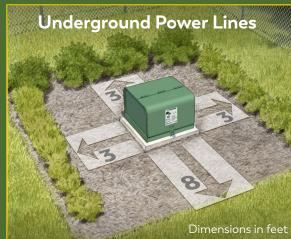
**Use this illustration** (above) as a guide for planting away from underground electric pad mount transformers. Planting away from transformers ensures they are accessible for inspection, maintenance, or repair. Don't assume underground lines aren't at risk from damage. Always contact MISS DIG 8-1-1 at least three working days prior to planting to have underground facilities marked.
